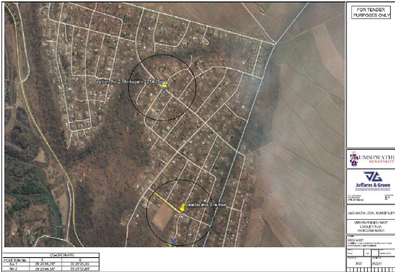
Figure 5: Positions of the High Mast Towers in Thokozane (Source: uMshwathi LM Town Planning Section)
